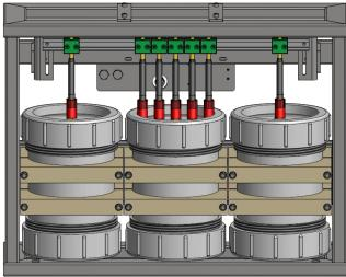
In the center of the frame there are three brackets that can hold two SFB1 battery packs and one SFC1 seafloor controller. Thanks to the cable management brackets all subsea connectors can be mounted stress free to guarantee correct operation.
